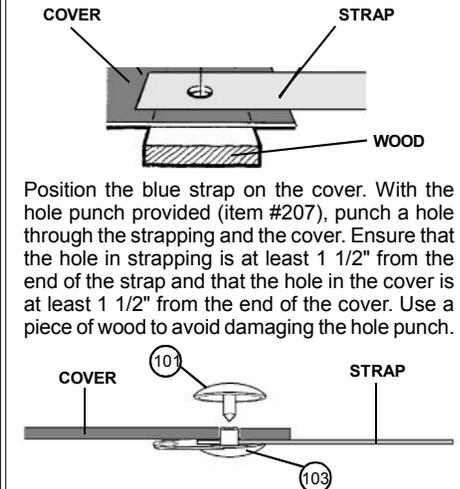
Insert female grommet (item #103) through hole in strapping and cover. Ensure that material is completely pushed down shaft. Insert male grommet (item #101) into female grommet. Once in place, hit gently with hammer until secure. (Caution - excess force will break grommet).
