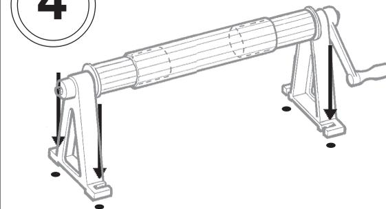
Using the two holes of the #4 A-frame (item #57) as guides, make two marks on deck for each #4 A-frame. With a 1/2" concrete drill bit, drill a 1 1/2" deep hole at each mark.
