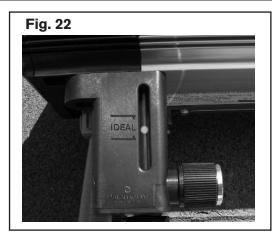
meter counter clockwise until the ball reads in the middle of the two lines on the flow meter. **(Fig. 22)**
