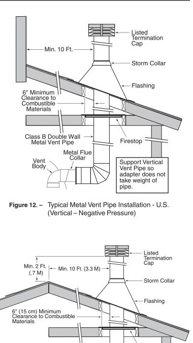
Figure 13. – Typical Metal Vent Pipe Installation - Canada (Vertical – Negative Pressure)
