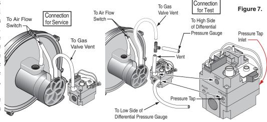
Do not attempt to adjust the gas input by adjusting the regulator setting. The correct gas regulator setting is required to maintain proper combustion and must NOT be altered.
