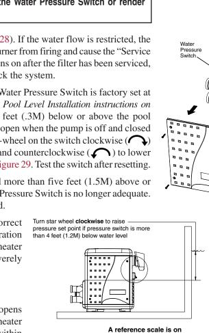
Turn star wheel **counterclockwise** to lower pressure set point if pressure switch is more than 5 feet (1.5M) above water level \_\_\_\_\_\_
