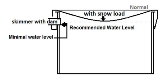
\Lower levels than this and the snow loading can damage the perimeter of the cover due to the excessive stress on the hem.
