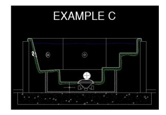
Example C is a hot tub which is on the floor slab. The tub is simply placed on the slab and a "skirt" is built up around the shell on the slab.
