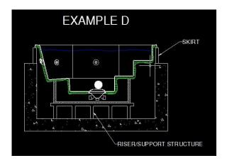
It is recommended that an access hatch is built into the pad under the stairs so a person may be able to access the underside of the tub for inspection/maintenance.
