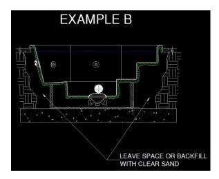
Example B is outdoor and in-ground. A concrete floor is poured for the tub, but no walls are poured and the floor slab would extend to the edges of the tub. The space under the tub may be left empty or back filled. If you choose to back fill install a barrier between the PVC fittings and the backfilled sand. This is to protect the fittings from being damaged by the pressure of the sand. Use clear sand is all cases.
