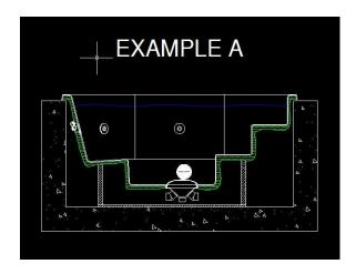
Example A is probably one of the most common methods of creating the concrete pad for new installations. It is in ground and has walls poured as well. This may also be similar when replacing an old concrete hot tub with a pre-plumbed acrylic shell where rather than pouring a pad the existing concrete shell is reused.
