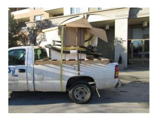
If a forklift is not available you will require 4-12 people to lift and move the hot tub to the final location. Another option would be to roll the hot tub on several pieces of 4'' piping.
